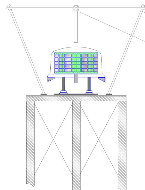
CONNECTORS HOLDING RING TO SUPPORT RODS SHOULD HAVE FLUSH MOUNTED FASTENERS AND HAVE ALL CORNERS ROUNDED
